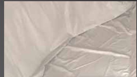
The liner is constructed of reinforced polyester fabric coated with PVC resin and is expected to last 30 years.
